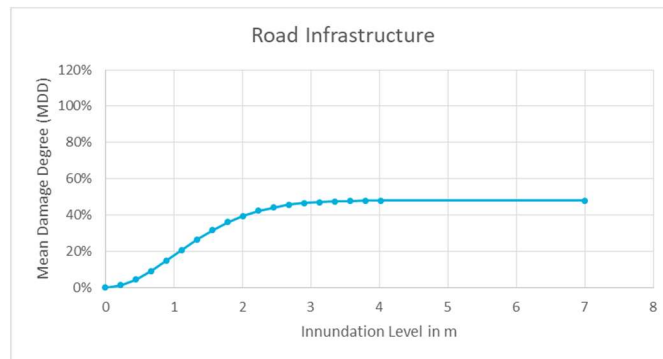
Figure 20 Damage function for the Road Network
