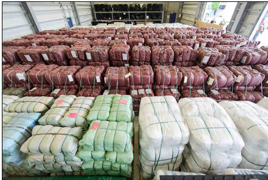
Figure 96: Example of a flood protection storage/warehouse. Bunks of sandbags can be stored until use against floods. Source: https://bit.ly/33Lkvb9 (02.03.2021).
