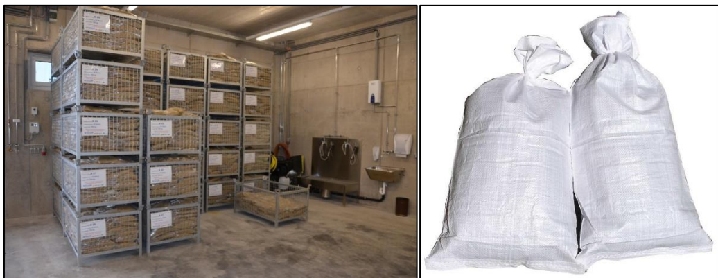
Figure 97: Example of a flood protection storage facility for sandbags (left). Example of polypropylene (PP) sandbags. Source: https://www.feuerwehr-neuhaus.bayern/kat-lager/ (02.03.2021).
